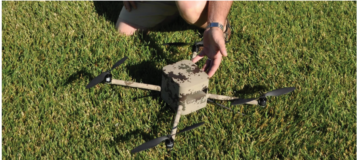
Leptron's RDASS 4 unmanned aerial vehicle weighs only five pounds
