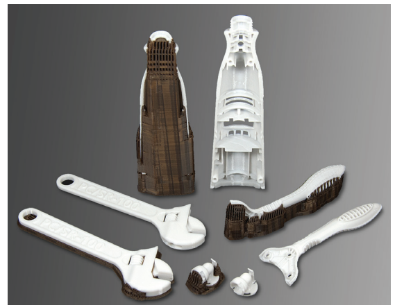
3D-printed models are shown with soluble support material (brown) intact, and after removal.
